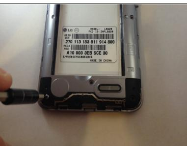
Once the back cover and battery are removed, use the Phillips #J000 screwdriver to remove all 11 screws located around the plastic midframe.
