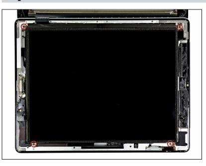
• Remove the four 2.0 mm Phillips screws securing the LCD to the rear case.
