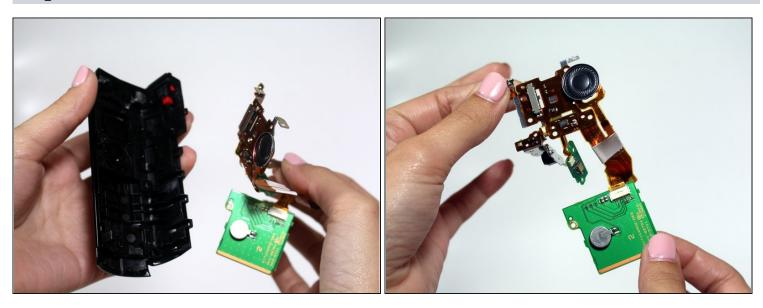
• Carefully pull the speaker out of the casing.
