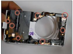
• Start by removing nine (4mm, PH00) of the screws which hold the outer silver trim bezels to the main chassis highlighted in red.
