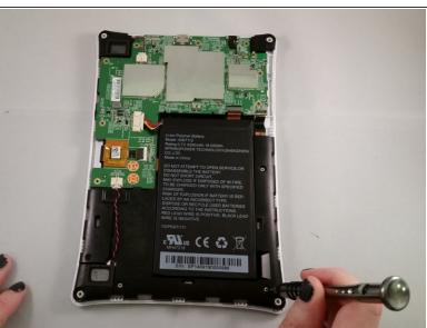
• Unscrew the circuit board from the motherboard by using a Phillips #0 screwdriver to unscrew the 4mm screws in a clockwise rotation.
