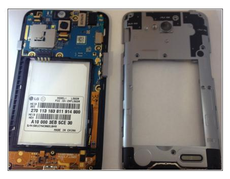
Using the plastic opening tool, carefully pry and separate the plastic midframe from the rest of the phone.
