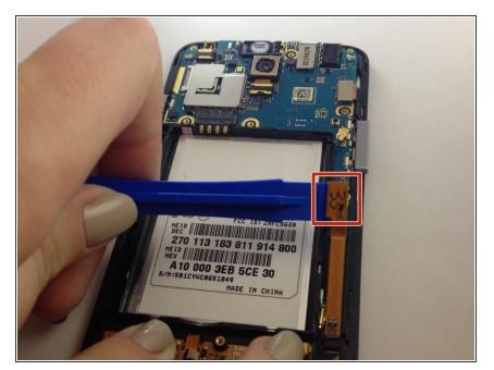
Locate where the motherboard connects to the orange sisterboard. Using the plastic opening tool, disconnect the connection between the phone and the orange ribbon cable.
