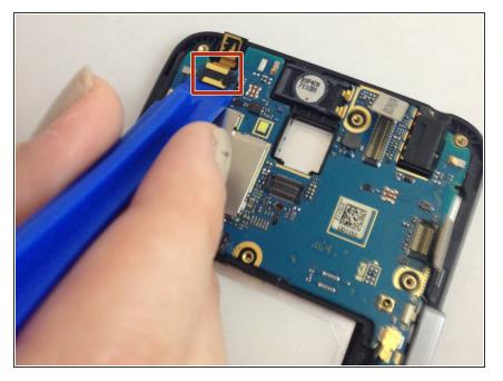
Locate the front facing camera in the top left hand corner of the motherboard. Using the plastic opening tool, separate the ribbon cable from the phone.
