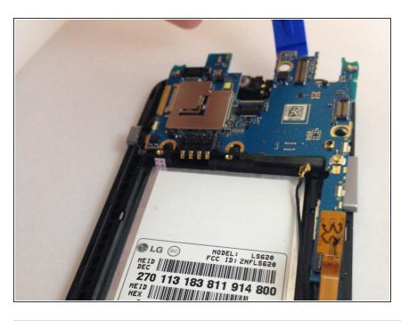
Using the plastic opening tool, carefully remove the motherboard from the phone.
