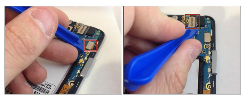
• Locate the ribbon cables in the top right corner of the motherboard. Using the plastic opening tool, remove the ribbon cables from phone.
