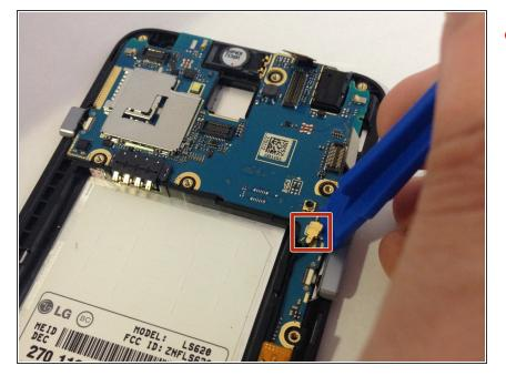
Using the plastic opening tool, disconnect the ribbon cable that connects the antenna to the motherboard.
