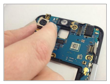
After removing the ribbon cable, the camera should be easy to remove with your fingers. Remove the rear facing camera.
