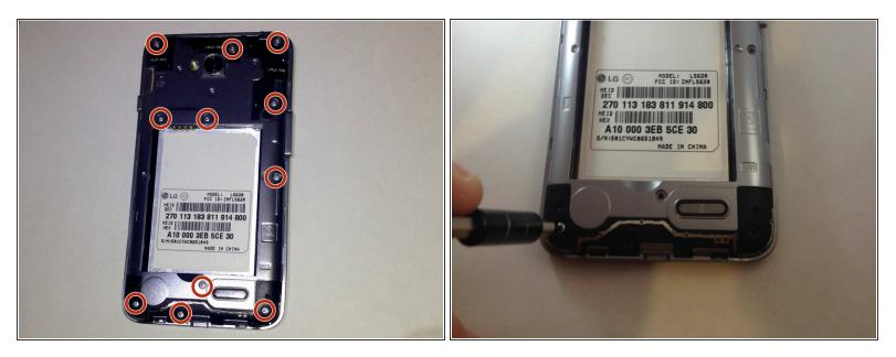
Once the back cover and battery are removed, use the Phillips #J000 screwdriver to remove all 11 screws located around the plastic midframe.
