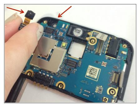
• After removing this ribbon cable, you will be able to easily remove the front facing camera with your fingers.
