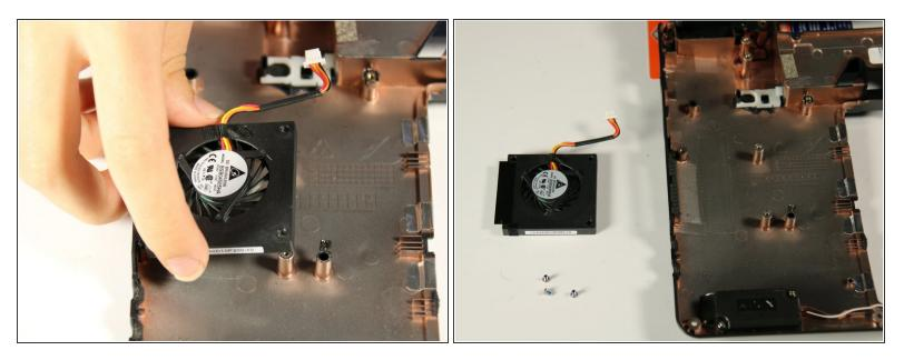
• When the 4 mm screws are removed, pull out the fan from the PC.
