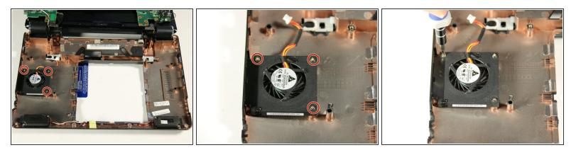
• Remove the three 4 mm screws that hold the fan down using a PH00 (+) Phillips head.
