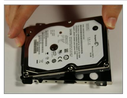
Remove the hard drive from the metal casing by lifting it up.
