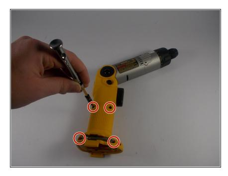
Using an H-5.0 bit driver remove the four T-10 Torx screws.
