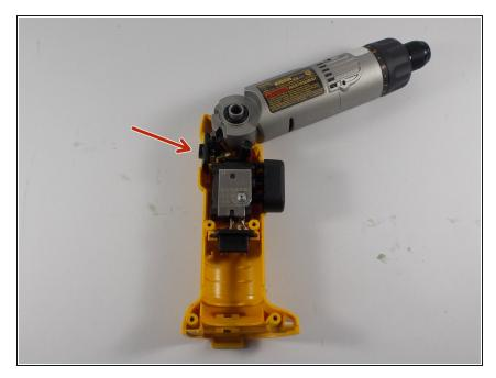
Locate the switch on the top of the drill right before the bending joint.
