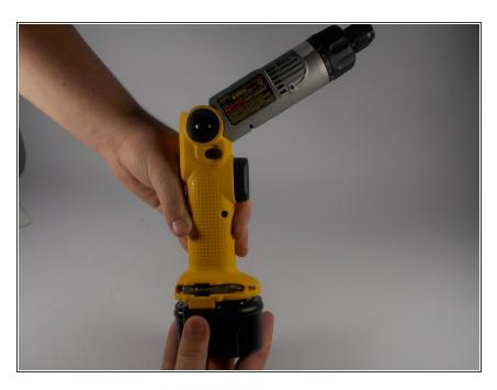
Firmly grip the handle of the drill with one hand and the battery with the other.
