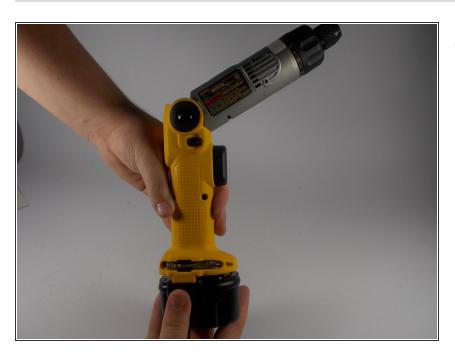
With the two tabs pushed in pull the battery out of the drill.
