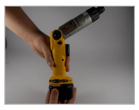
Using the hand holding the battery press the two tabs that are located on the left and right side of the battery where it connects to the drill.
