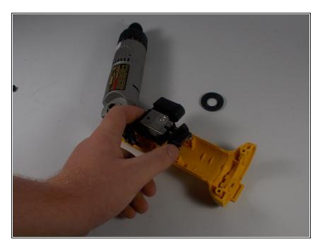
Gently lift the broken trigger assembly out of the slot.
