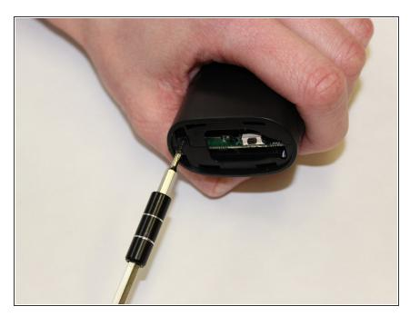
Use the metal screwdriver to unscrew the screw from the back of the device.
