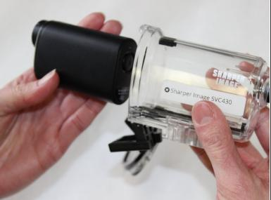
Once the latch is free, simply pull the front of the waterproof case off and slide the camera out.
