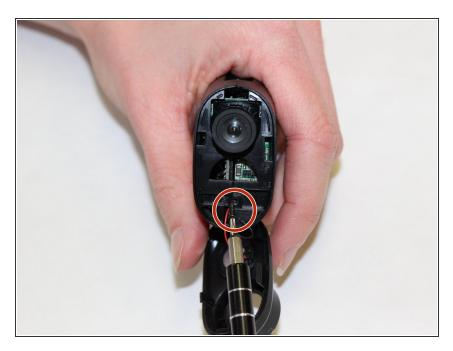
Using the screwdriver, unscrew the screw located underneath the front panel.
