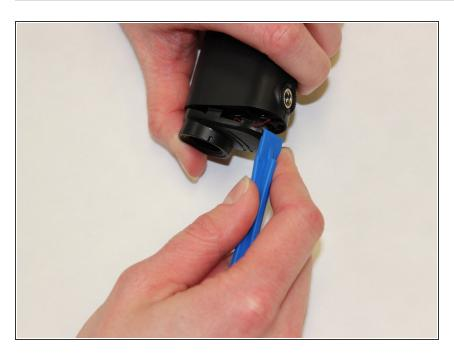
Use the plastic opening tool to pry off the front panel of the device.
