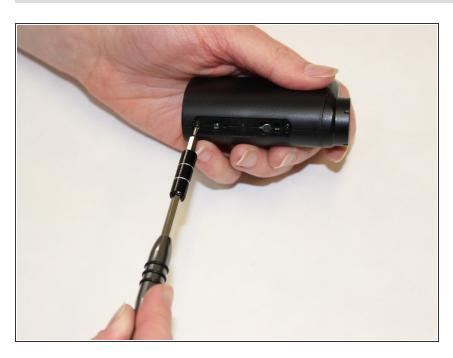
Use the JIS J0 screwdriver to unscrew the two screws on the top of the device.
