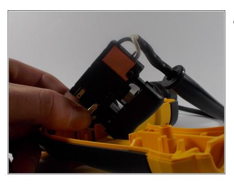
Disconnect the last wire from the trigger box using the same method from the previous step.
