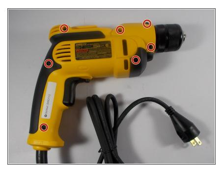
Remove seven TR20 Torx Security screws from the side of the drill.
