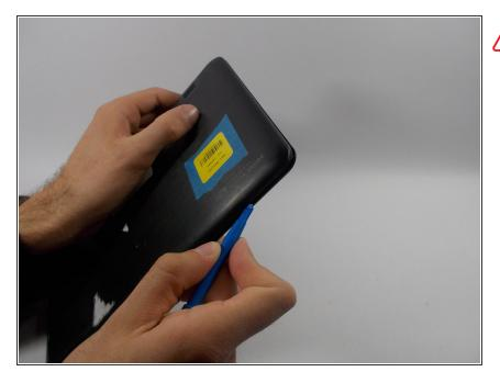
Please be aware that removing the rear panel from the back of the Flex 10.1 may cause damage to the rear panel.
