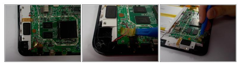
• Using the plastic opening tool or your fingers, remove the tape holding the black and red wires down.
