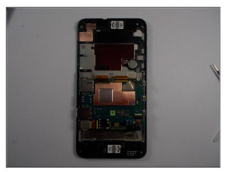
Once you have removed the wire, you can carefully lift up the motherboard
