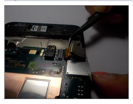
Carefully peel off the adhesive so that the camera can be disconnected from the mother board
