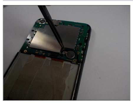
With your pair of tweezers carefully unplug the black and red wire in order to remove the motherboard
