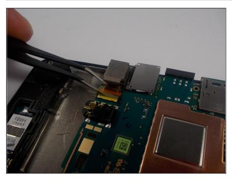
Peel off the yellow film that's attaching the camera to the motherboard
