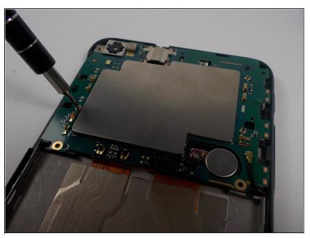
• Take the PH000 screwdriver head to take out the one screw that's holding down the green panel. (The screw is located on the left side of the panel)
