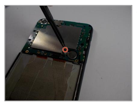
With a pair of tweezers disconnect the battery wire from board.
