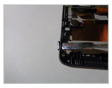
Using a metal spudger, push the power button out gently.
