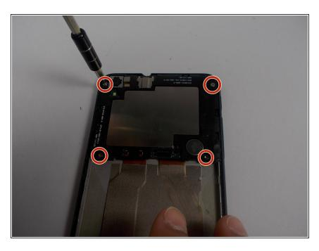
Using the T5 screw driver, unscrew the four screws that are holding down the black plastic casing.
