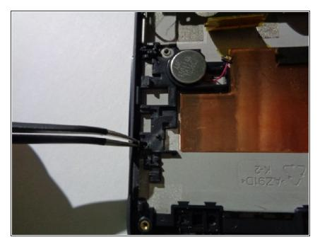
Using the a pair of tweezers, locate the rubber button piece and gently lift up in order to set it free.
