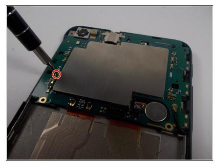
Using the PH000 screw driver, unscrew the remaining screw that is holding down the motherboard. It is located on the left side of the motherboard.
