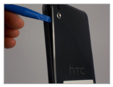
Pry open the back panel by inserting the plastic opening tool on the left of the camera. We find this spot the easiest to get the tool under the panel.
