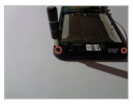
Using the T5 screw driver, unscrew the following screws.
