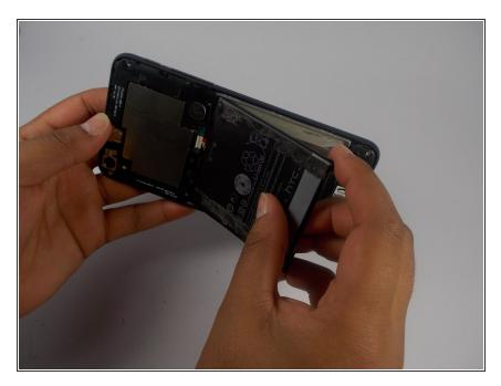
Carefully lift battery backside first to disconnect the white connector.
