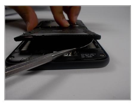
There is adhesive on the other side of the battery as well, take the nylon spudger used to get off the panel and cut through.
