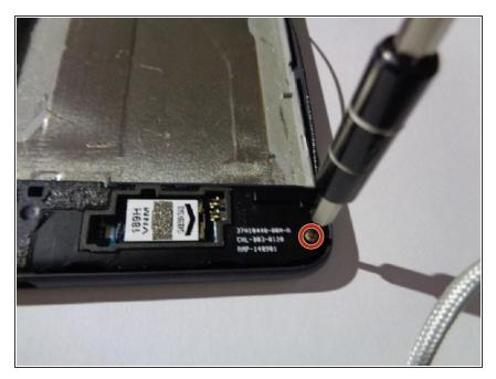
Using the T5 screw driver remove the remaining screw at the bottom right corner of the phone.
