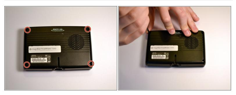
• Remove the four 4.2 mm screws on the back cover of the device using a Phillips #0 screwdriver.
