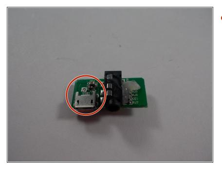
Once board is removed, locate silver component on the board. This is the charging port. Remove the charging port. To put it back on the board you need to solder the component back onto the board.
