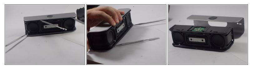
• Grab two metal spudgers and insert one into the slit underneath the silver plating on the top of the device. Pry upward with the spudger until you unhook the two locks on the top. Repeat same step for the bottom of the device. When all four tabs are released, slide device out of the casing
