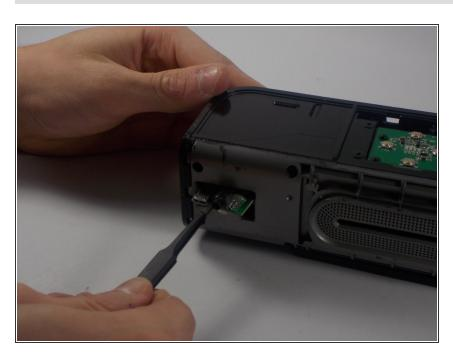
Remove the circuit board containing the aux port using the tweezers.
