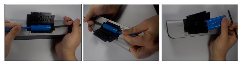
• Use the nylon spudger and the plastic opening tool to lift up the battery from the casing. Use the spudger on one side and the plastic opening tool on the other.
