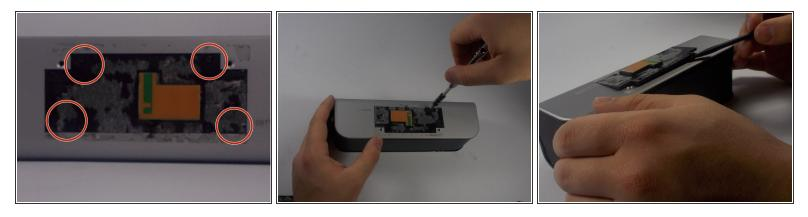
• Unscrew the four 6mm screws located under pad using the PH0 screwdriver head and lift plastic cover using the nylon spudger. Be careful not to sever the wire that leads to the circuit board.
