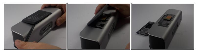
• Remove the rubber pad from the bottom of the device by using the nylon spudger to pry the glue holding it together. Then use the spudger to remove the rubber pad.
