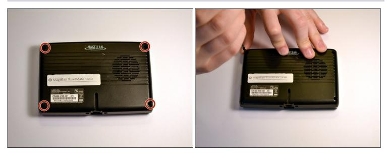
• Remove the four 4.2 mm screws on the back cover of the device using a Phillips #0 screwdriver.
