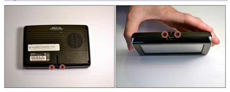
• Remove the two 4.2mm screws at the bottom of the device using a Phillips #0 screwdriver.
