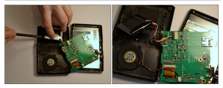
• Use the black spudger to break the seal between the adhesive and battery. Use the same spudger to continue to pry the battery from the backing
