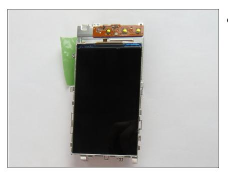
The LCD screen is now separated form the main frame.
