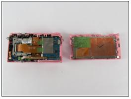
Separate the LCD half compartment of the camera from the main body.
