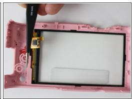
Use the tweezers to pull out the home and playback buttons from the camera frame.
