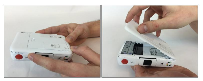
Push the rear face plate from the short side nearest the screws you just removed towards the other short side of the camera. It should slide forward and unlock the clips holding it in place.
