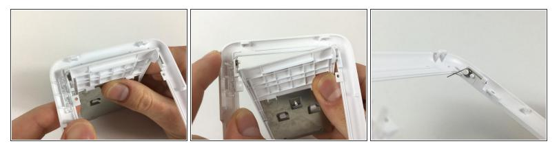
• Maneuver the plastic paper door out of the sockets one at a time. Make sure to be gentle so the plastic does not snap. Also, make sure to keep track of the small springs.
