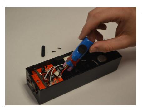
Remove the ICR18650-26M battery from its position by pulling upwards and out of the casing.
