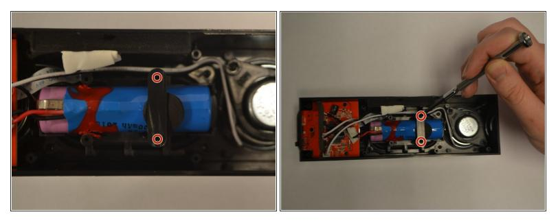
Identify the two Phillips (Length-5/16", Head-1/8") screws holding the battery in place and remove them using a #1 screwdriver.
