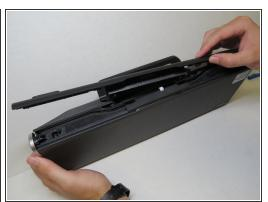
Use the plastic opening tool to run along the outside edges of the speaker. Pry along the seams
