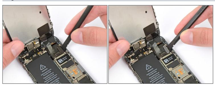
• Use a spudger or a fingernail to disconnect the front-facing camera and sensor cable.
