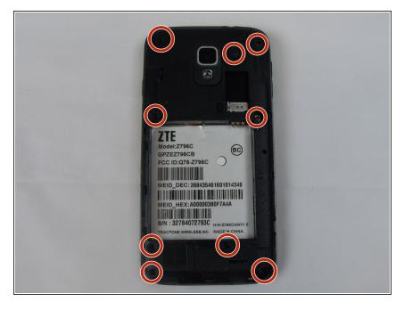
Remove the back of the phone by removing the 9 PH000 shown
