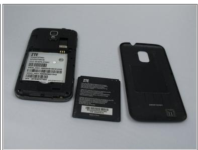
Pry the battery out of the groove in the phone with your finger.
