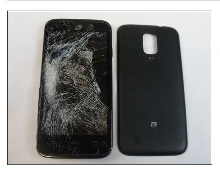
Using either your finger or a plastic opening tool, pry the back off to reveal the battery.
