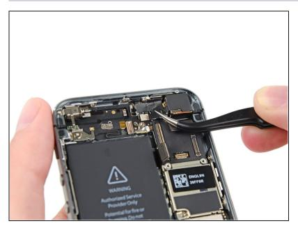
Remove any tape covering the camera flash bracket.
