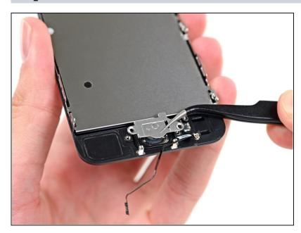
Remove the home button bracket from the display assembly.
