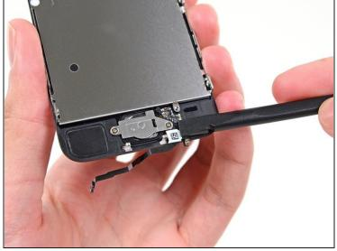
• Fold the home button cable down, out of the way of the home button bracket.
