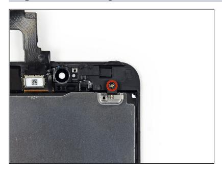
Remove the 2.7 mm Phillips #000 screw from the back of the display assembly.
