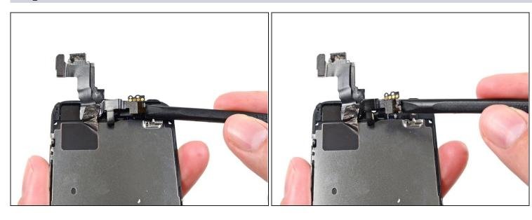
• Use the flat end of a spudger to gently peel the front-facing camera portion of the cable away from the display assembly.
