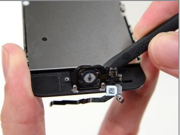
Peel the home button the rest of the way off of the display by prying gently with a spudger.
