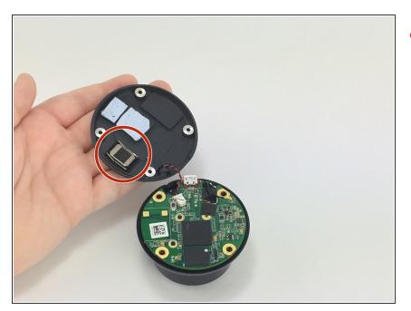
• Open the back panel completely to expose the speaker indicated by the red circle.
