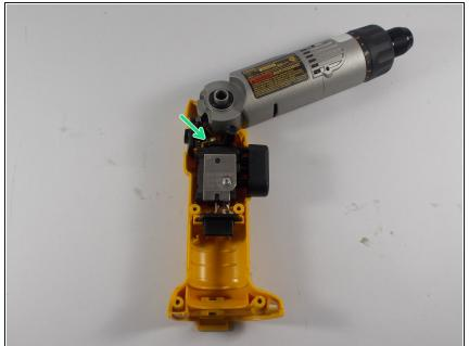
Carefully release the connection between the rotational switch and the motor assembly. This should be done carefully to ensure that the switch connection switch on the assembly is not damaged.
