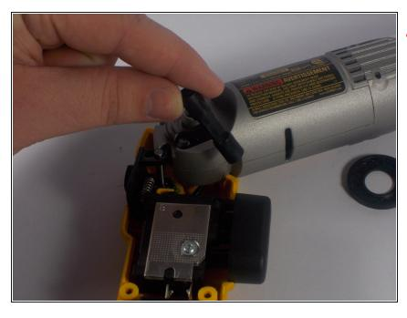
♠ Once the switch is freed from the assembly, firmly grip it between two fingers and lift it straight out of the drill frame.
