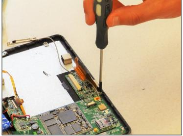
• Locate the four 5mm screws holding the motherboard in place and remove them using the Phillips #0 Screwdriver.
