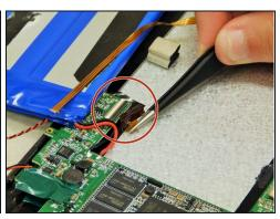
Carefully remove the remaining ribbon cables using the tweezers. Make sure that all ribbon cables are detatched before attempting to remove the motherboard.
