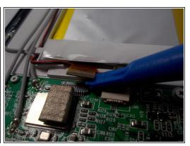
Disconnect the ribbon cable from the motherboard by lifting up on the connector.
