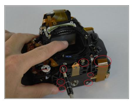
Several screw and ribbon cables and the bottom portion of the camera need to be removed as shown in the picture
