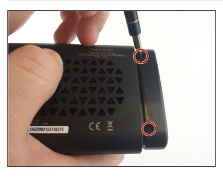
Remove four (4) 11.7 mm Phillips #0 screws from each side at the bottom of the speaker.
