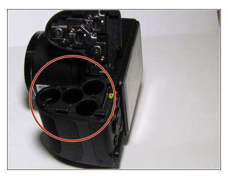
• When all of the batteries have been removed you should see four places for four new batteries to be inserted
