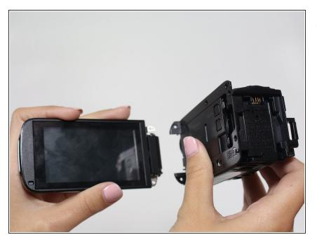
• Remove the LCD display from the camera body.
