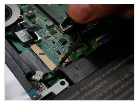
Using the tab on the cables connector with your hand unplug the Hard Drive connection cable and remove it from the cable track on the battery.
