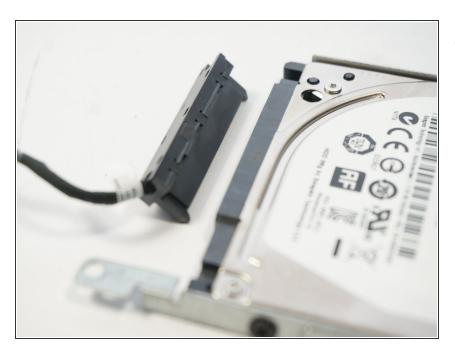
Unplug the adapter cable from the drive. No tool is required for this step.
