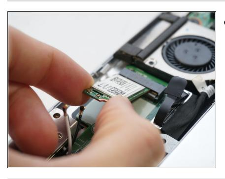
Lift the wireless card upwards and remove.
