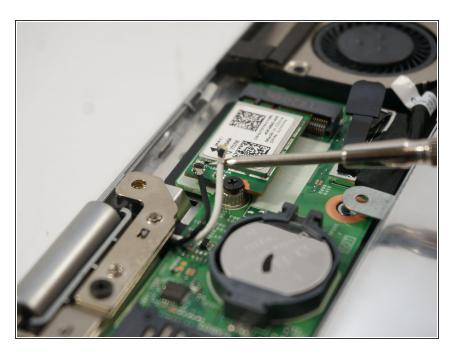
Detach the wires connected to the wireless card.
