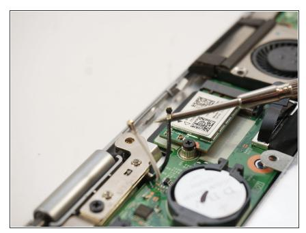
Ensure both wires are detached from the piece.
