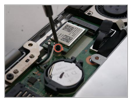
Remove the single 3mm screw holding down the hardware using a plastic Philips Head #0 Screw Driver.
