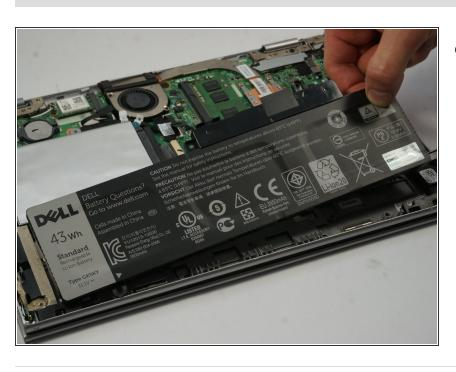
Once the screws have been removed the battery may then be simply removed by hand and replaced.
