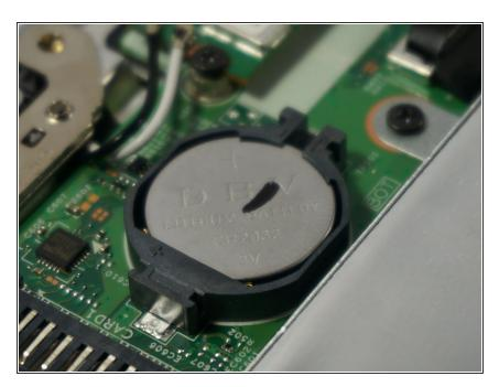
Using a plastic spudger, gently press under the battery to lift it up and out.
