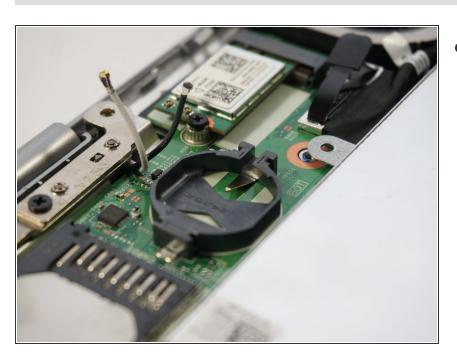
Remove the CMOS Battery
