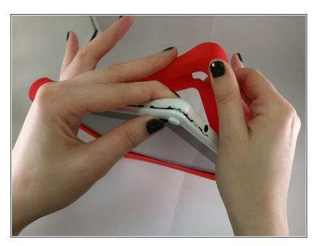
Remove the red rubber case from the device.
