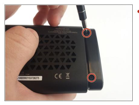
Remove four (4) 11.7 mm Phillips #0 screws from each side at the bottom of the speaker.
