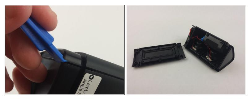
• Use the plastic opening tool on one of the corners to separate the bottom piece from the speaker, and then remove the piece.
