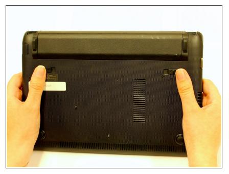
Hold the laptop using both hands with the battery facing upwards.
