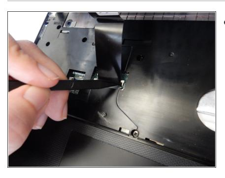
Using the spudger push the white clips upwards that are holding the cable.
