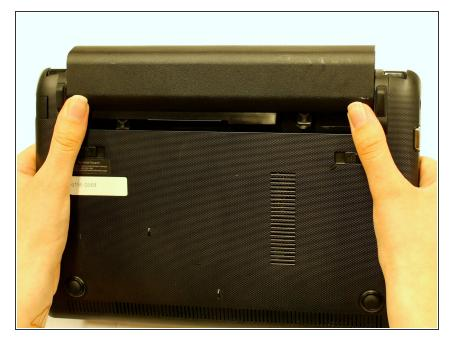
Push the battery upwards and out of the laptop as shown.
