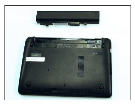
Continue to push the battery upwards until it is completely separated from the laptop as shown.
