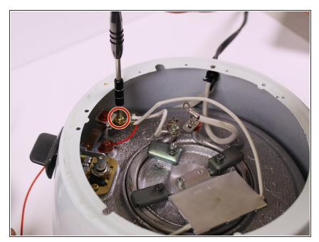
Remove the 7mm Phillips screw that connects two white wires and one red wire to the heating "warm" switch.
