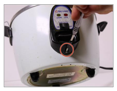
Remove the 11mm Phillips screw from below the power component panel.
