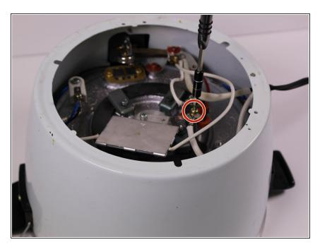
Remove the 7mm Phillips screw holding the white and maroon colored wires that are connected to the heating element.
