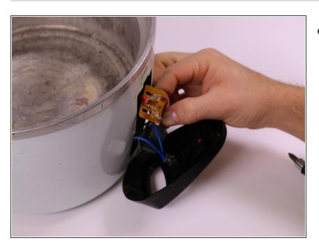
Pull the light plate from the power component panel.
