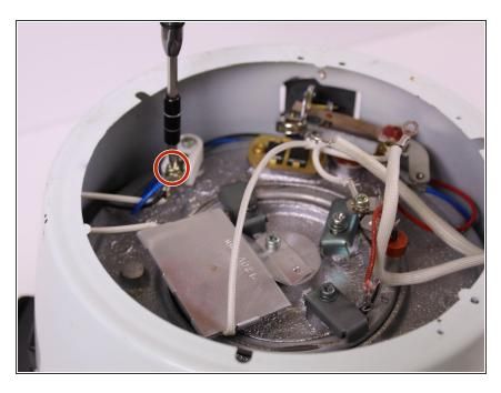
Remove the 10mm Phillips screw that connects the white, blue and black wires to the white plastic piece in the corner of the device.
