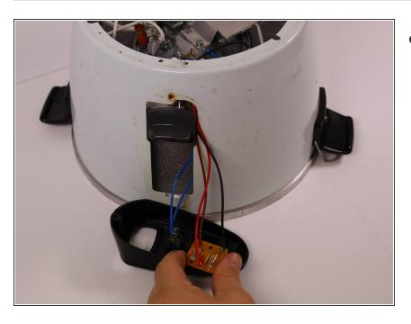
Using your hand, pull out the light plate with the maroon red and black wires.
