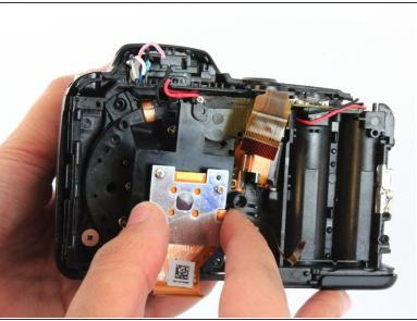
Remove the three 1.5x2.5mm screws using a PH000 screw head.
