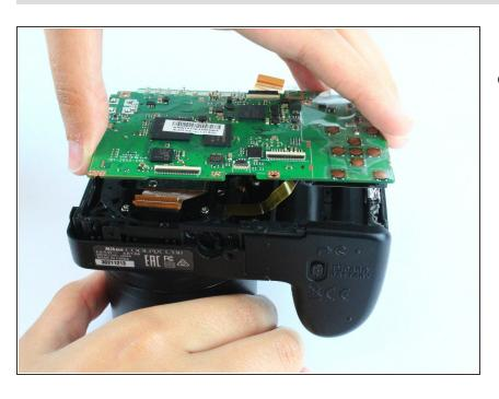
Remove the motherboard by lifting it directly up.
